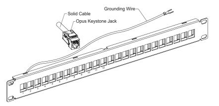
Expand the Foldable Wire Management Grip, hook the grips into fixture at both ends of the patch panel. Fix the solid cables to the cable fixture hole by cable ties.
