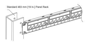
Position the cable assembled RJ45 module from back of panel and then snap in the RJ45 modules into the RJ45 window all the way down until the latch on module is locked to panel as shown in Figure. Follow the installation in sequence until all required RJ45 modules are installed.
